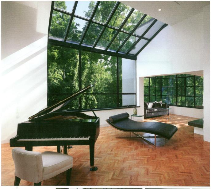
Guests often are treated to cocktails and music at the studio, now used as a private art gallery. Restoration involved welding new columns around the originals, repairing the concrete spiral stair, and reinforcing the water-damaged chicken-wire floor deck with steel.
